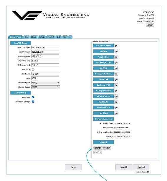
It is possible to update the firmware in the encoder using the Update Firmware button, only update with files sourced from Visual Engineering. Follow the procedure described on screen to complete the update.
