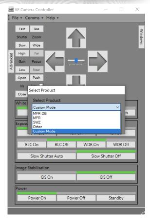
If connecting to the camera using TCP/IP enter the IP address and port of the camera in the application settings panel.
