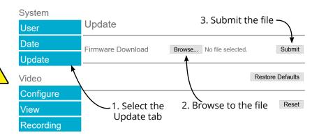
Following a **Submit** the camera will update the firmware and display the following text: Programming in Progress...Do NOT remove power
