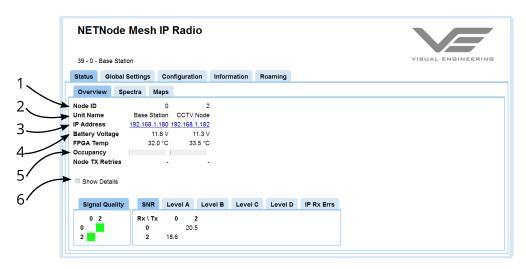
This displays detailed status information of received signal quality and enables navigation between nodes. The Status tab is divided into three sub-tabs:
