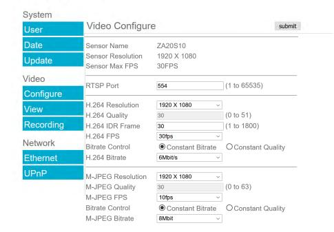
The Video page contains parameters for each encoder type. The encoder has two fundamental modes of operation:
