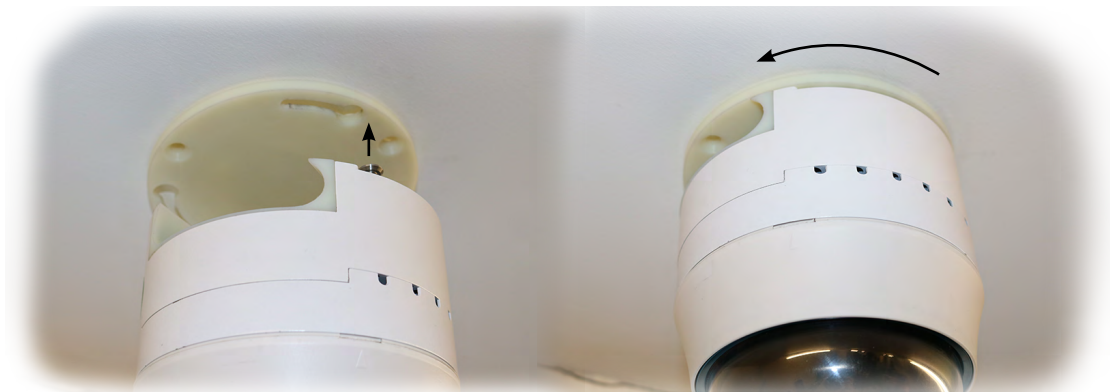
Camera offered to plate, lugs aligned to mount.
