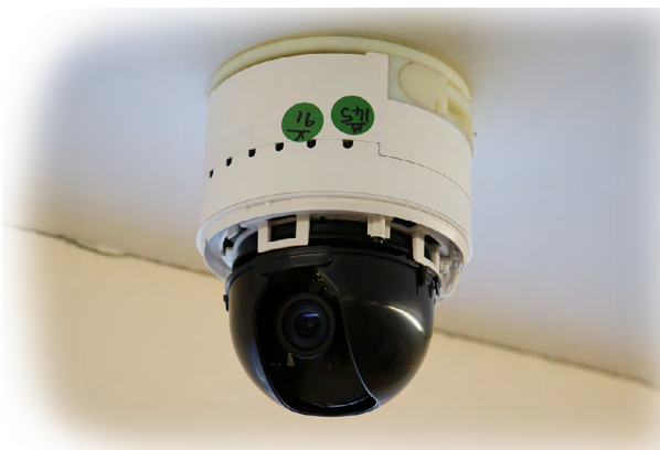
External dome removed
